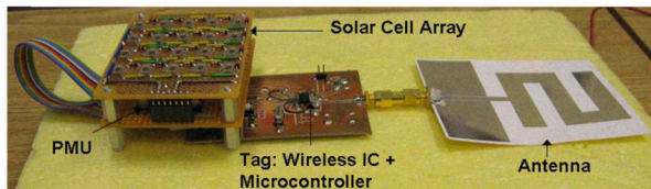
Fig 6. Working Prototype of Solar Powered battery-less Tag.
