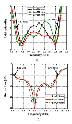
Fig. 6. Dependences of (a) axial ratio and (b) return loss of the omnidirectional CP antenna on the length of the conducting cylinder.
