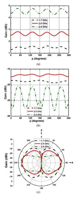
Fig. 3. Simulated gain patterns for the omnidirectional CP antenna: (a) LHCP in the horizontal plane (i.e., the xy plane); (b) RHCP in the horizontal plane (i.e., the xy plane); (c) LHCP in the elevation plane (i.e., the xz plane).
