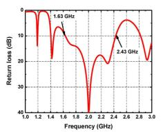
Fig. 2. Simulated return loss for the omnidirectional CP antenna.
