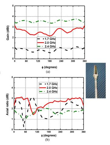
Fig. 13. Measured gain and axial ratio patterns for the omnidirectional CP antenna in the omnidirectional plane (i.e., xy plane): (a) gain pattern; (b) axial ratio pattern.
