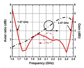
Fig. 4. Simulated axial ratio and gain averaged in the omnidirectional plane for the omnidirectional CP antenna.
