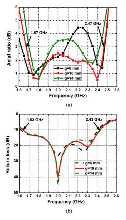
Fig. 7. Dependences of (a) axial ratio and (b) return loss of the omnidirectional CP antenna on the gap length of the conducting cylinder.
