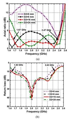
Fig. 5. Dependences of (a) axial ratio and (b) return loss of the omnidirectional CP antenna on the diameter of the conducting cylinder.
