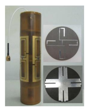
Fig. 9. Prototype of the broadband omnidirectional CP antenna with front and back views of the feeding network.
