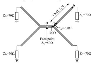
Fig. 8. Equivalent circuit for the feeding network of the omnidirectional CP antenna.
