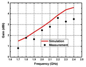
Fig. 12. Measured gain for the omnidirectional CP antenna compared with simulation result.
