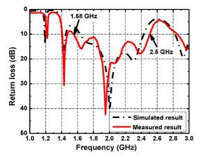
Fig. 10. Measured return loss for the omnidirectional CP antenna compared with simulation result.
