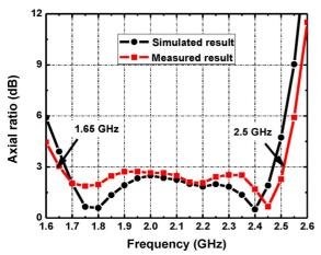
Fig. 11. Measured axial ratio for the omnidirectional CP antenna compared with simulation result.
