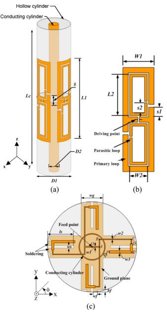
Fig. 1. Configuration of a broadband omnidirectional circularly polarized (CP) antenna: (a) perspective view; (b) broadband cp element; (c) feeding network.
